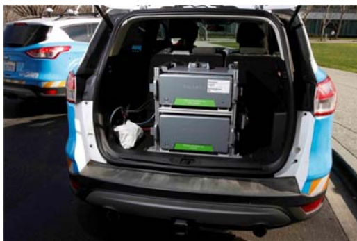
Figure 3—Picarro analyser and computer onboard a PG&E survey vehicle
