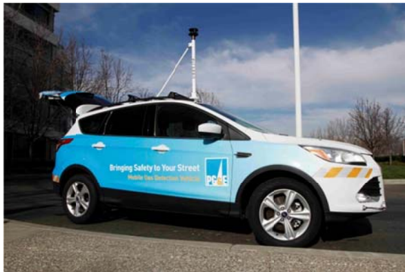
Figure 2—PG&E Picarro leak detection survey vehicle
